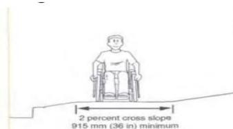
**GOOD DESIGN** A level area at least 915 mm (36 in) wide improves access when the street elevation is lower than the building elevation
