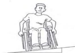
**PROBLEM** Wheelchair users traveling on a sidewalk with a cross slope greater than 2% use more energy to to offset the force of gravity that directs them towards the curb and into the street
