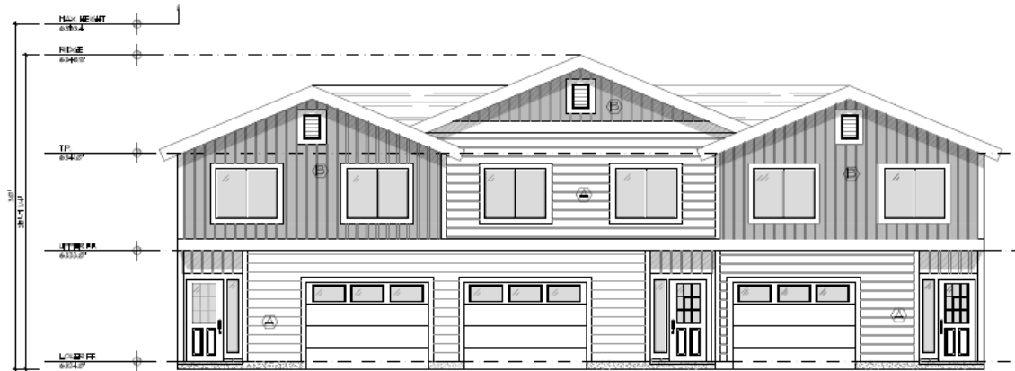
① TRIPLEX CONCEPT - A FRONT ELEVATION Scale: 1/4"=1'-0"
